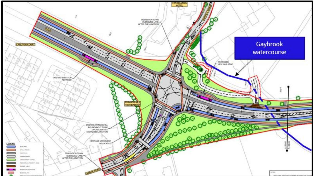
Figure 4.11 Proposed works at Pinnock Hill Roundabout and R132 (around Ch. A00 +250)
